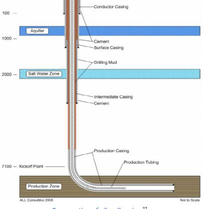
Cross section of oil well casing 27
